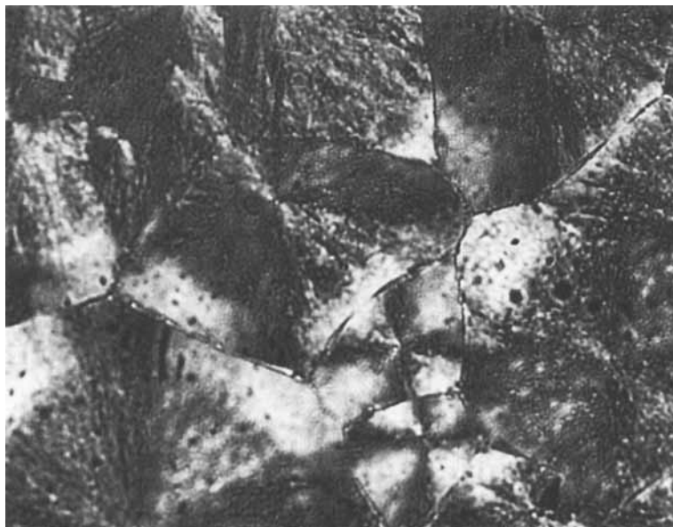
FIGURE 3 Microphotograph of anhydrous HDPCl in mesophase showing fan-like texture at 90°C 55x.
